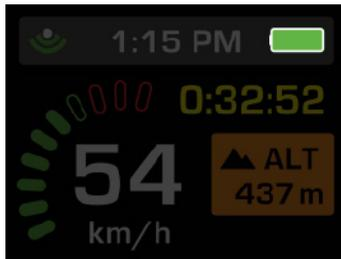
When Transcend has partial battery power it will be represented by a variation of the following icons, located in the top right hand corner of the display at all times.
