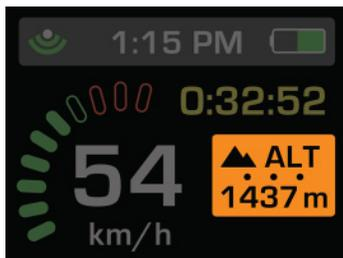
Transcend calculates altitude by measuring air pressure which changes as you move up and down with elevation. In addition, air pressure is constantly changing due to changing weather. To compensate for this, Transcend uses GPS to automatically
