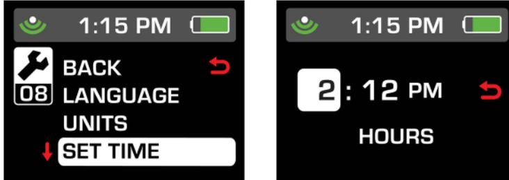
Transcend utilizes Coordinated Universal Time (UTC) upon first strong GPS signal lock. This allows the clock to automatically calculate the proper Greenwich Mean Time (GMT). However, you may have to set the correct hour based on your time zone. A table is provided below to aid you.
