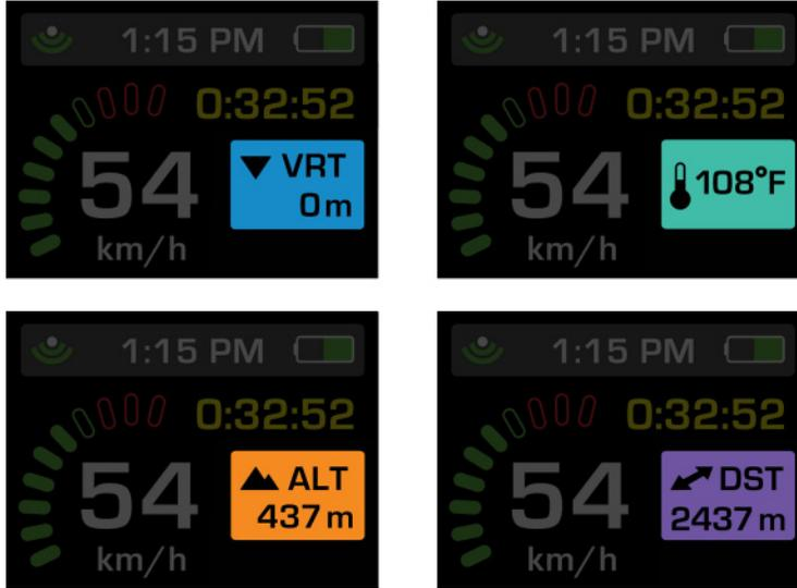
Transcend offers a configurable dashboard that allows you to choose one of the following Features to be displayed alongside the permanent Features of the main dashboard screen. The default feature viewed is *Current Altitude*.
