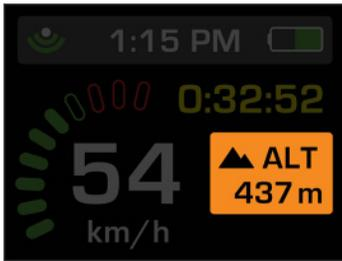
Transcend's Dashboard has a customizable function as well. There is a coloured square area in the bottom right-hand corner of the screen where you can choose to see another feature of your choice along with the Speedometer, Stopwatch/Chrono and Status Bar. The default feature is Altitude, see 'Setting the Configurable Dashboard Feature' to learn more.
