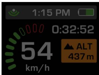
Pressing SELECT while viewing the Dashboard will activate Chrono/Stopwatch mode, the numbers will turn yellow and start counting until you press SELECT a second time.
