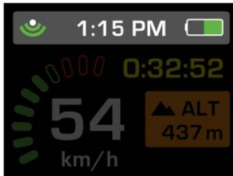
Across the top of the screen are three important pieces of information at all times. This Status Bar appears in all screens and menus and provides the vitals of Transcend: GPS Indicator, Time, and Battery Indicator.
